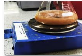
Figure1. Reduction of silver nitrate by sodium citrate and the appearance of a yellowish-brown color in the AgNO 3 indicated the formation of silver nanoparticles.
